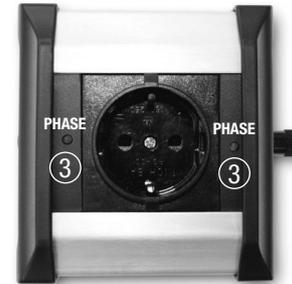
Should the same LED ③ light up even after you have turned the plug through 180°, make a connection with the enclosed earth cable between the PHASER ④ and the earth of the device to be tested. The outside contact of a Cinch socket, for instance, makes a perfect earthing point.
