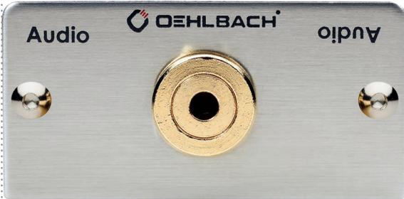
Audio multimedia tray with high-quality breakout cable. A 3.5 mm audio-jack socket is located on both sides of the multimedia tray. The tray comes with 24-carat gold-plated contacts. In combination with the mounting frame, any two multimedia trays (alternatively one tray combined with a blind cover) may be used for each frame with the internal dimensions of 50x50 mm.
